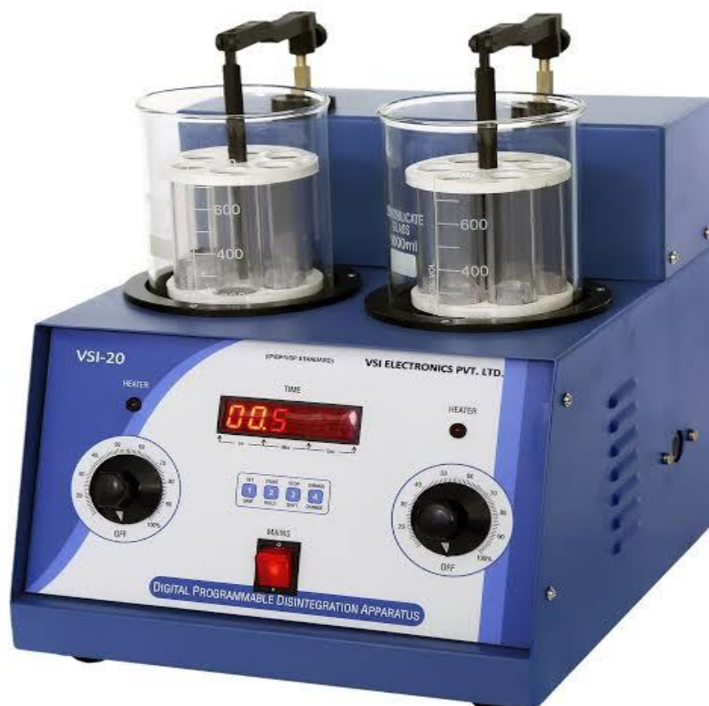
Figure 5: Disintegration test apparatus
