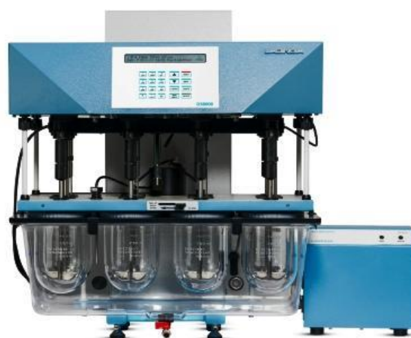
Figure 6: In vivo Dissolution test apparatus
